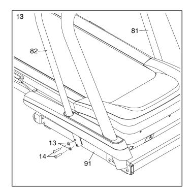
14. Firmly tighten the two 5/16" x 1 1/2" Patch Bolts (15).
